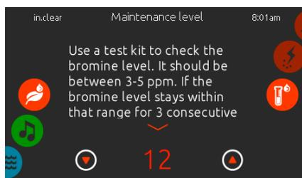
*If you do, retest the bromine level the day after. If the bromine is not in the 3-5 range and is higher than 5 ppm, decrease the maintenance level. If the bromine is lower than 3 ppm, increase it. Repeat until the test reads a bromine level in the 3-5 range.*
